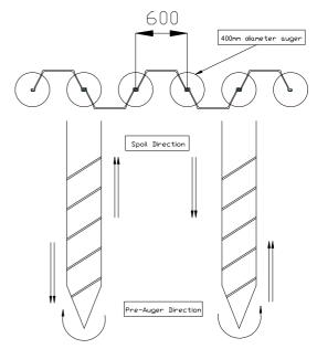
When pre-augering we drill-in in one direction and we counter rotate the auger whilst extracting it to return as much of the disturbed ground to its original position as possible. We do not wish to create voids in the ground and we do our utmost to avoid doing so.
